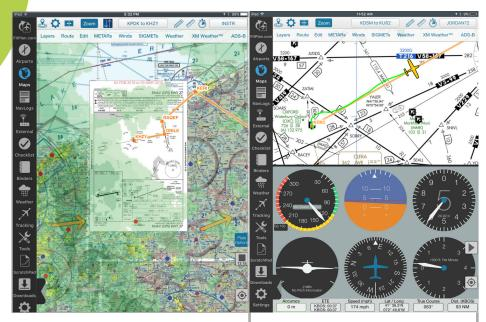
View approach plates over Weather, METARs, and Winds on a map. Adjust the transparency for clear viewing of the base map layer. This feature allows for rubber-banding so that the route of flight can be aligned with the approach path.
